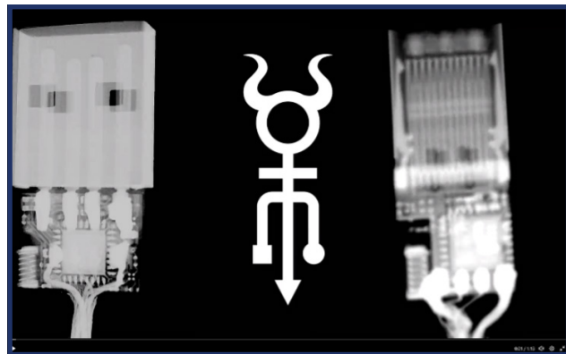
Figure 12 Connector with embedded chip (From the video of O.MG adapter maker Twitter)
